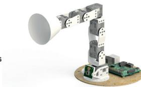
**a servomotor** is the combination of an engine and an electronic card performing precise control (servo motor in a position, speed or given force).
